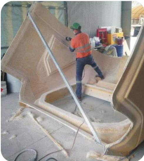
**Downer EDI Rail and Bombardier** – Static and live simulator manufacturing and installation. Prototyping of train interior and locomotive fronts.
